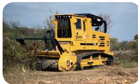
Predator Mulcher Head Uses Variable Displacement Motors to Maximize Productivity
