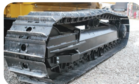
Heavy Duty Undercarriage with 2-Speed Drives
