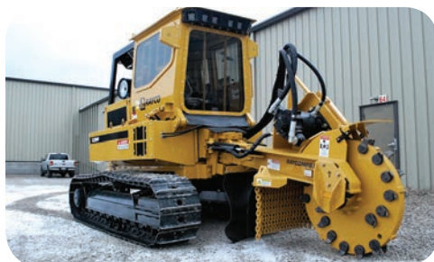
40-inch x 3-inch Cutter Wheel ith 36 Monster Tooth Cutter Tools
