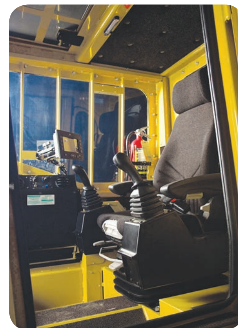
Forestry Cab with Rooftop Escape Hatch and Heated, Suspension Seat
