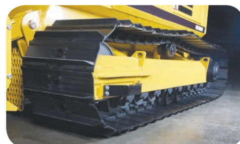
Heavy Duty Undercarriage with 2-Speed Final Drives
