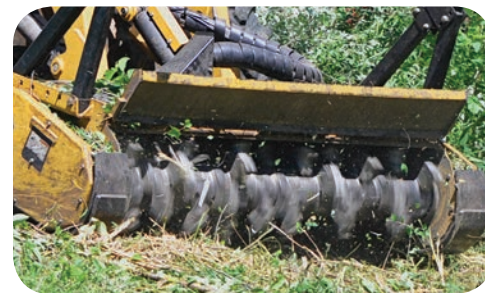
Predator Mulcher Head with Dual Drive and Variable Displacement Motors.
