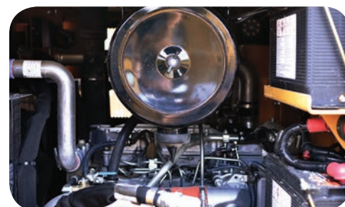
Powerful 200 hp Isuzu Diesel Engine and Reversing Fan
