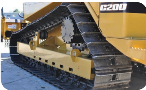
EASY CLEAN - Hi-Track Steel Undercarriage with 2-Speed Travel
