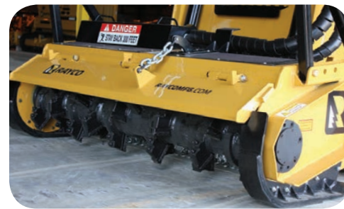
Predator Mulcher Head with Variable Displacement Motor
