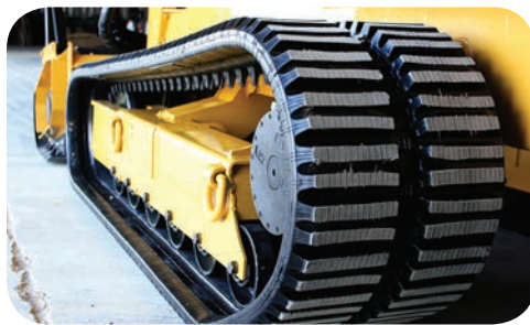
Rubber Track Undercarriage with 2-Speed Travel
