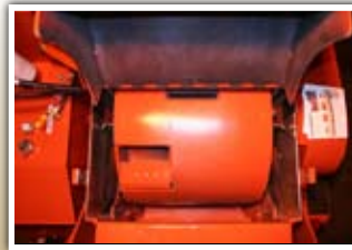
DRUM/AIR IMPELLER SYSTEM 36" diameter, 6-knife staggered pocket drum with twin, 4-blade air impeller system
