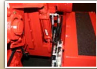
HYDRAULIC DOWNFORCE Variable Force Hydraulic Down Pressure System creates 600 lbs. of perpetual down pressure
