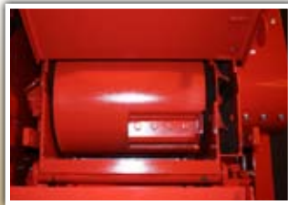
DRUM 21" diameter, 8-blade, chambered air-impeller system
