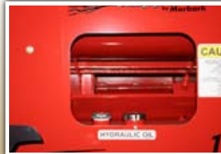
SELF-CONTAINED HYDRAULIC SYSTEM PTO models are equipped with a self-contained hydraulic system
