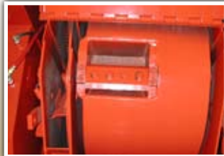
DRUM/AIR IMPELLER SYSTEM 36" diameter, 4-knife staggered pocket drum with 36" diameter, 8-blade chambered air impeller system
