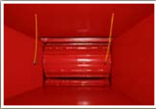
TORQMAX FEED WHEEL TorqMax Top Feed Wheel Compression System with 3:1 torque amplification
