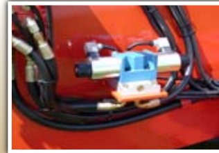
REVERSING AUTOFEED Reversing Automatic Feed System reduces wear and increases knife life
