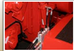
HYDRAULIC DOWNFORCE Variable Force Hydraulic Down Pressure System creates 700 lbs. of perpetual down pressure
