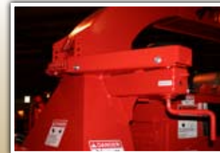
DISCHARGE CHUTE 360° Manual Crank Swivel Discharge with infinite rotation
