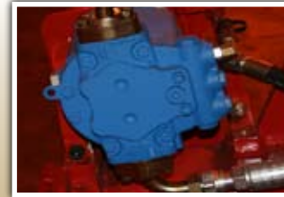
HYDROSTATIC DRIVE 2.5ci hydrostatic motor with .4ci functions gear pump, 16cc track drive gear pump and 4.6ci hydrostatic transmission
