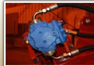
HYDROSTATIC DRIVE With 4.6 ci hydrostatic motor, .5 ci gear pump and 2.5 ci hydrostatic transmission
