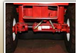
ARTICULATING FRONT AXLE Maintains stability on uneven terrain
