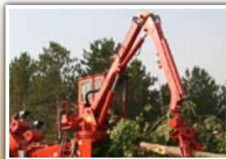
LOADER OPTION The Morbark 500 knuckleboom loader allows for the chipping of whole trees and a variety of wood waste.
