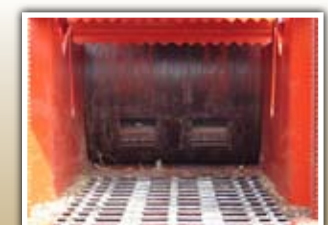
FEED WHEEL Close positioning of the feed wheel to the anvil provides constant down pressure.
