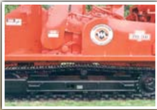
UNDERCARRIAGE CAT 312B undercarriage provides 18" ground clearance, while an optional skidder-style blade stabilizes the unit on steep grades.
