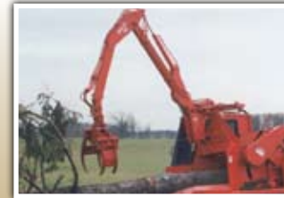
LOADER The Morbark 150 knuckleboom loader allows for the chipping of whole trees and a variety of wood waste.
